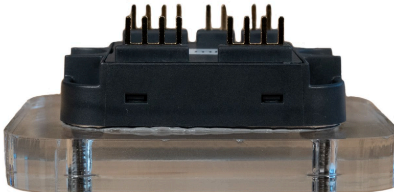
Figure 24: Thermal grease applied with an 8 mil stencil: large amount of thermal grease appearing around the side of the module, indicating excessive thermal grease application
