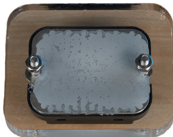
Figure 19: Thermal grease applied with a 4 mil stencil: module baseplate surface not fully wetted indicating insufficient thermal grease application
