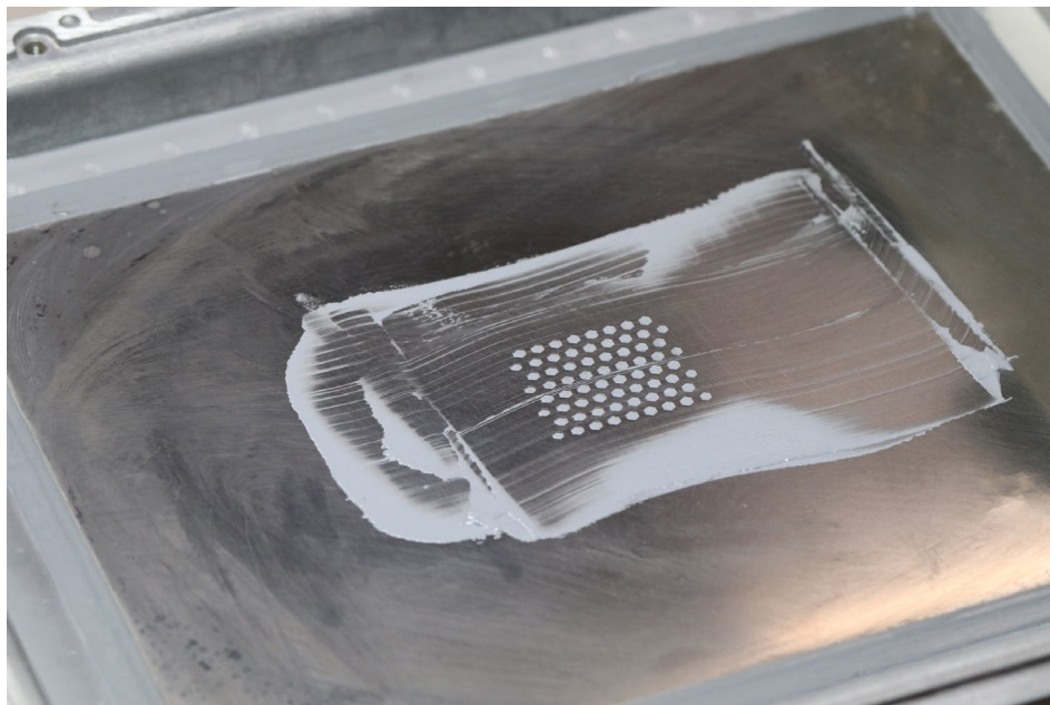
Figure 17: Correct application of TIM to stencil
