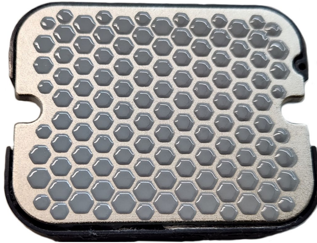
Figure 18: Correct application of TIM to DM power module
